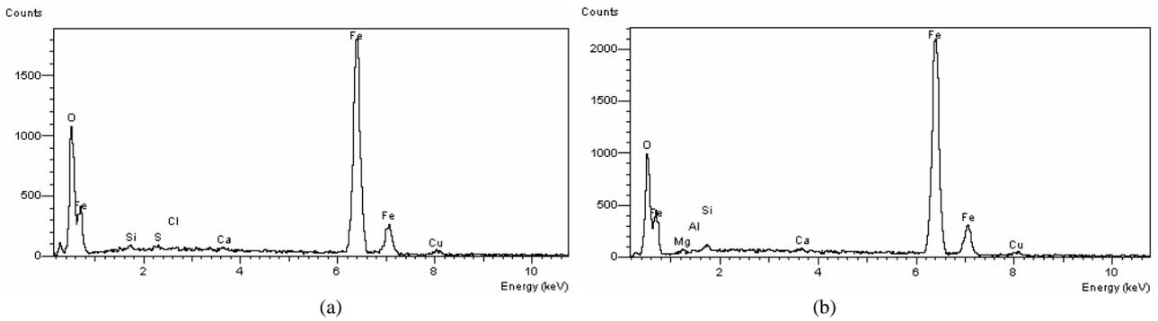
Fig. 3. EDS analyses of corrosion products obtained from different locations of the failed tube: (a) outer surface; and (b) inner surface.
