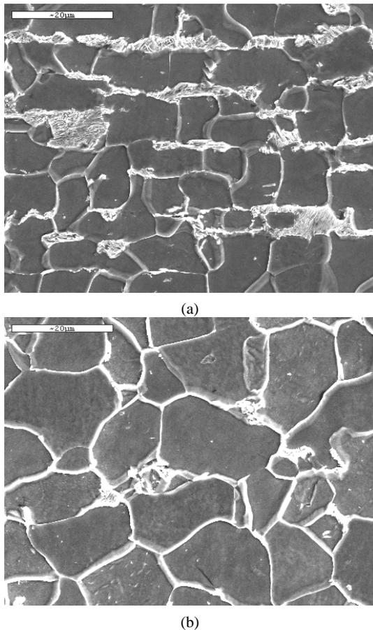
**Fig. 2.** Cross-sectional SEM micrographs of the economizer tubes: (a) new tube; and (b) failed tube.
