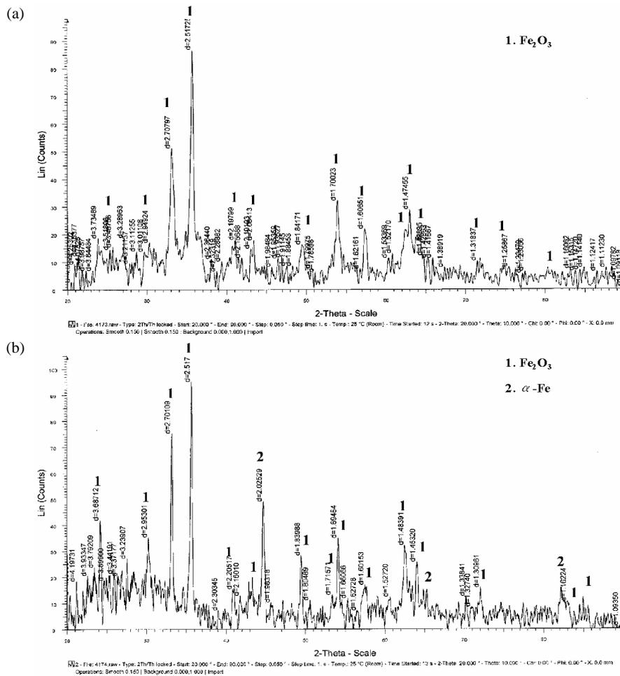
Fig. 4. XRD analyses of corrosion products obtained from different locations of the failed tube: (a) outer surface; and (b) inner surface.
