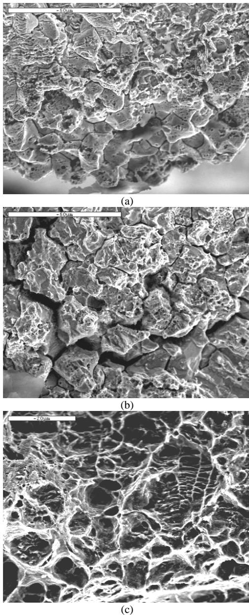
**Fig. 6.** SEM micrographs at higher magnification for: (a) spot A; (b) spot B; and (c) spot C, as designated in Fig. 5(b).
