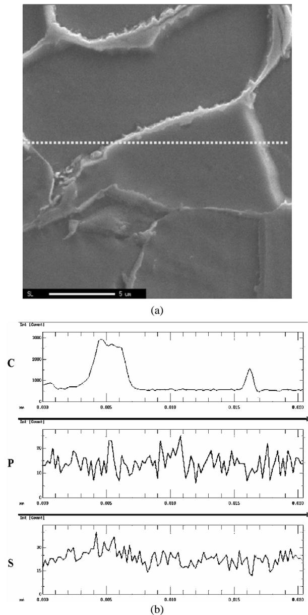
**Fig. 7.** EPMA line scanning analysis of failed tube: (a) SEM micrograph; and (b) C, P and S content distribution along the yellow dotted line in Fig. (a).
