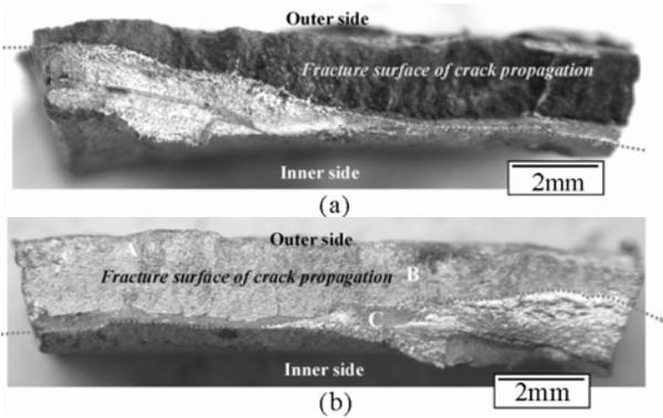
**Fig. 5.** The fracture surface appearance of the failed tube: (a) before descaling; and (b) after descaling.
